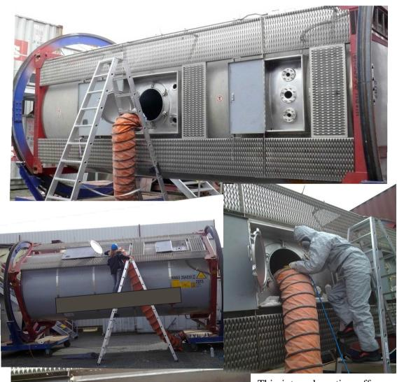
This internal coating offers protection against acid, lye, solvents up to several hundred °C.
