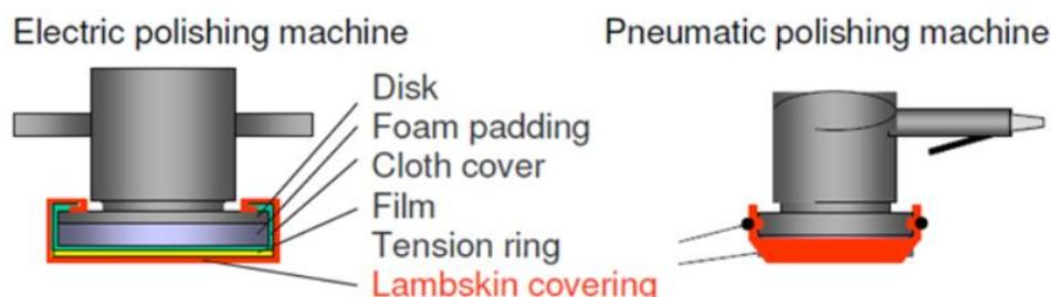
Charge the center of the lambskin covering with ca. 2 ml of **NewPro permaSeal CARE 150** and apply the material with the running machine without additional pressure to an area of approx. 0,5 – 1 m<sup>2</sup>.
